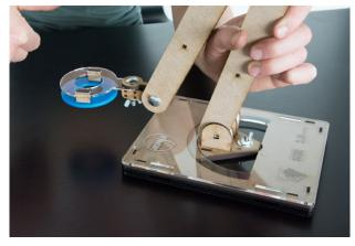
7.9 Insert a M5  $\times$  45 bolt so that its head is on the side with the square hole (invert components D1 and D2 if the wing bolt is not on the same side as the others). The metal washer and the wing nut are placed on the other side for fastening the assembly.
