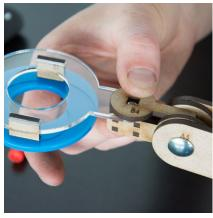
7.5 Insert a M5  $\times$  30 bolt so that its head is on the side with the square hole. The metal washer and the wing nut are placed on the other side for fastening the assembly.
