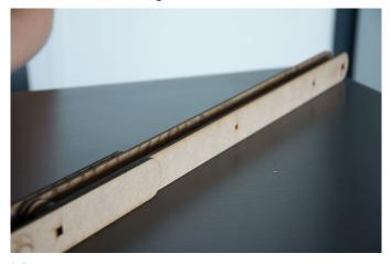
4.6 Insert the bolt so that its head is on the side with the square hole. The metal washer and the wing nut are placed on the other side for fastening the assembly.
