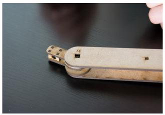
7.3 Insert a M5  $\times$  30 bolt so that its head is on the side with the square hole. The metal washer and the wing nut are placed on the other side for fastening the assembly.
