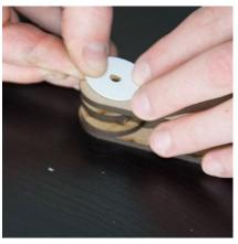
4.5 Place the end of the short arm with the "middle assembly" inside one of the ends of the long arm, at the level of the holes next to the logo. Take care that the square holes in the short and long arms are both located on the same side. This enables all the wing nuts to be on the same side where adjustment of the stand can be made.
